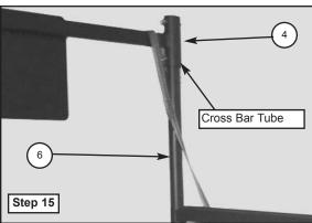
16. Using a 9/16" open end wrench and 9/16" socket and ratchet, attach the Cross Bar (4) to the two Swing Arm Posts (6 and 7) with four Hex Head Capscrews, 3/8-16x2-1/2" (1) and four Locknuts, 3/8-16 (3).
