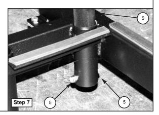
8. Attach the Left Hand Swing Arm Post Assembly (7) to the Frame left Outer Tube on the left side in the same way as described in steps 5, 6, and 7 above.
