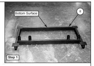
2. Using a 9/16" socket and ratchet and a 9/16" open end wrench, attach a Caster (9) to the Frame (8) with four Hex Head Cap Screws, 3/8-16x1" (2) and four Locknuts, 3/8-16 (3).
