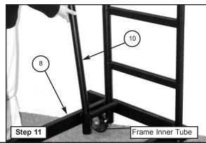
12. Using a 9/16" open end wrench and 9/16" socket and ratchet, attach the Back Rail Support Post (10) to the Frame Inner Tube with two Hex Head Capscrews, 3/8-16x2-1/2" (1) and two Locknuts, 3/8-16 (3).
